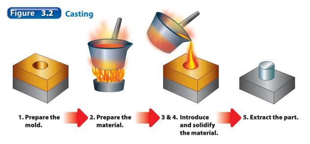
Liquid to Solid Molten metal, glass, clay, or plastic material takes on the shape of the mold as it cools. *What items do you use at home or school that might have been made by casting?*
