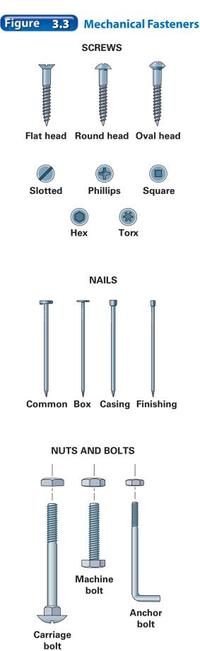
**Building Supplies** Screws, nails, nuts, and bolts are all mechanical fasteners. *Are all of these fasteners used for items that can be taken apart? Why or why not?*
